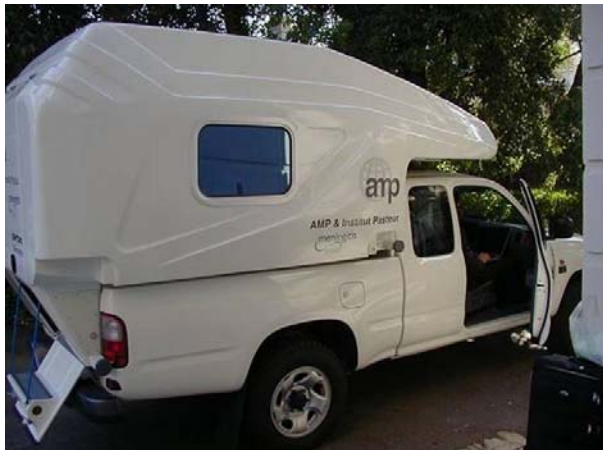
Figure 5: Mobile Laboratory 2. Note the lack of fixed solar panels and the detachable laboratory unit
