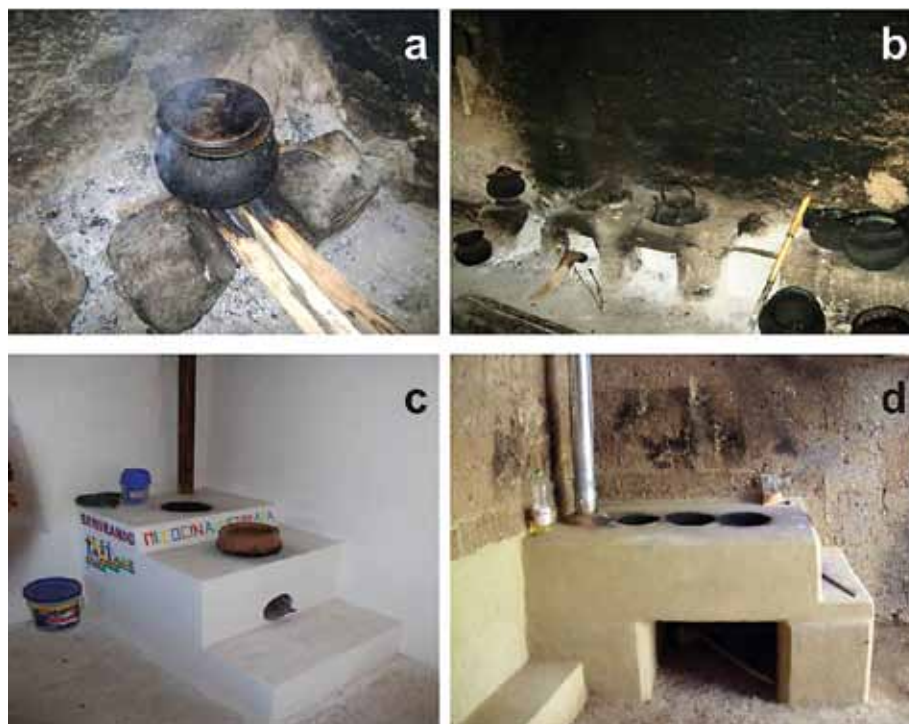
Figure 1. Type of stoves found in the Province of San Marcos and the OPTIMA-II improved chimney stove model. a: Open fire “Tulpia”; b: “Traditional” stove; c: government design “SEMBRANDO” stove; d: OPTIMA-II stove.
