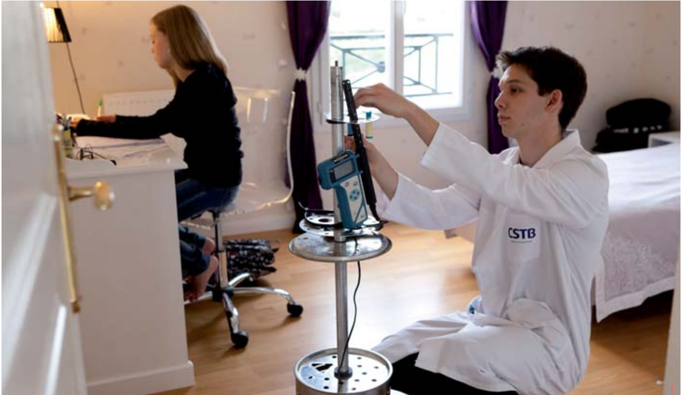
Indoor air quality measurement in a private home - ©OQAI-CSTB
