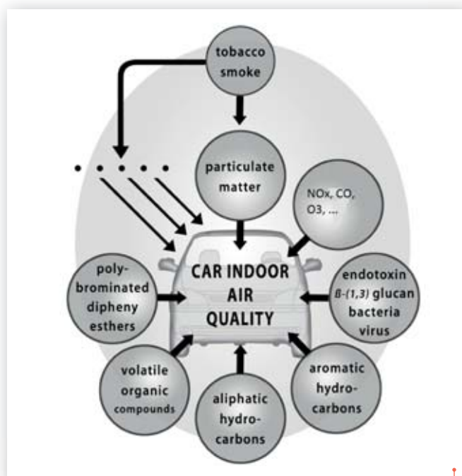
Figure 1- Common pollutant types found in car cabins (on the basis of Muller et al. (2011) [18])
