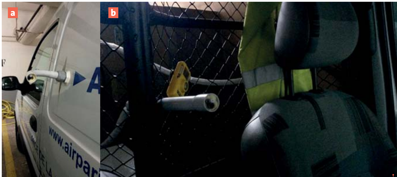
Figure 2 - Outdoor (a) and indoor (b) probes used for pollutant concentrations measurement © Amine Mehel
