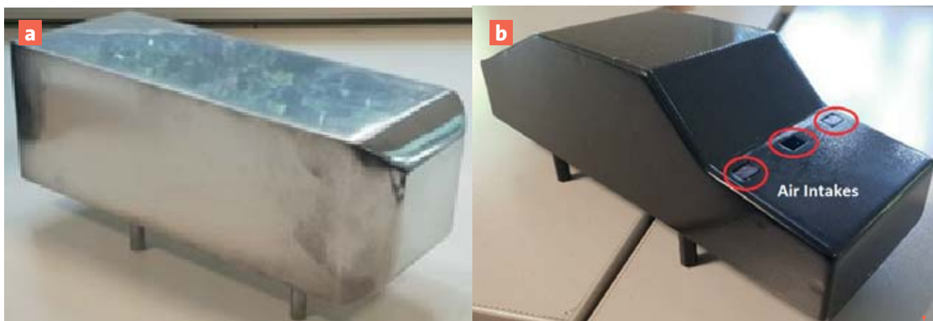
Figure 3 - Car models used for infiltration study: (a) Ahmed body, (b) Mira model © Amine Mehel
