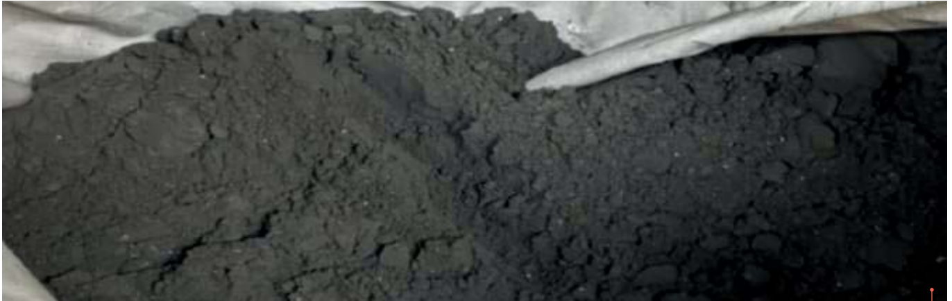
“Black mass” extracted from the grinding of battery cells, containing mainly a mixture of carbon, nickel, lithium and cobalt - ©Veolia
