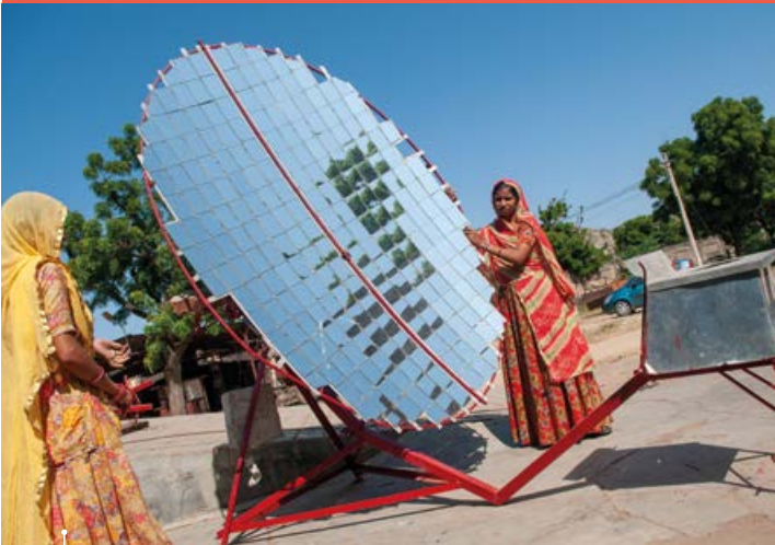
Tilonia, Rajasthan, India, 6 September 2011: Women constructing solar cookers at the workshop of Barefoot College in Tilonia, Rajasthan, India.
