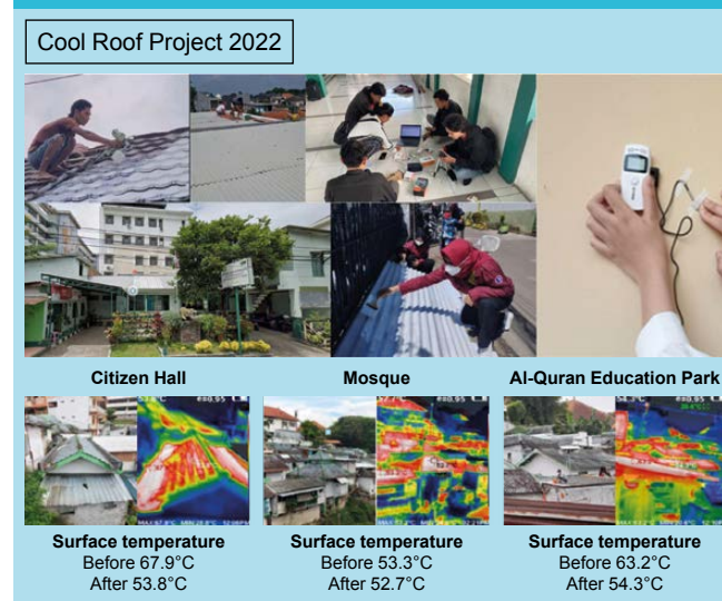
Figure 8: Cool Roof Project led in 2022: Pictures and results in surface temperature
